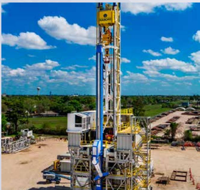
**Figure 1.** The electrical robotic pipe handler during field testing. Image provided by Nabors.
