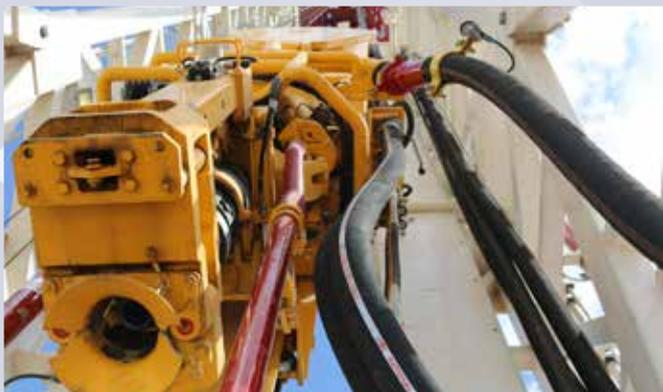
**Figure 2.** The TDS-11SAE is powered by two new 600 hp induction motors, increasing power for use in ERD wells. Image provided by NOV.
