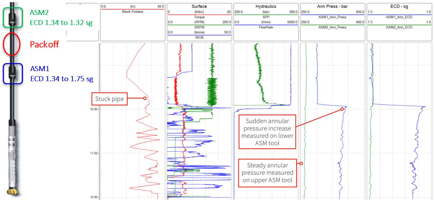
**Figure 2** – This time-based log shows measurements acquired by the BlackStream ASM tools placed along the drillstring. The sudden annular pressure increase indicated by the ASM tool closer to the bit (ASM1) was not seen on the ASM tool placed in upper part of the drillstring (ASM2). This data provided a clear picture of the wellbore condition and enabled Total E&P Norge AS to make an informed decision as to where to cut the pipe.
