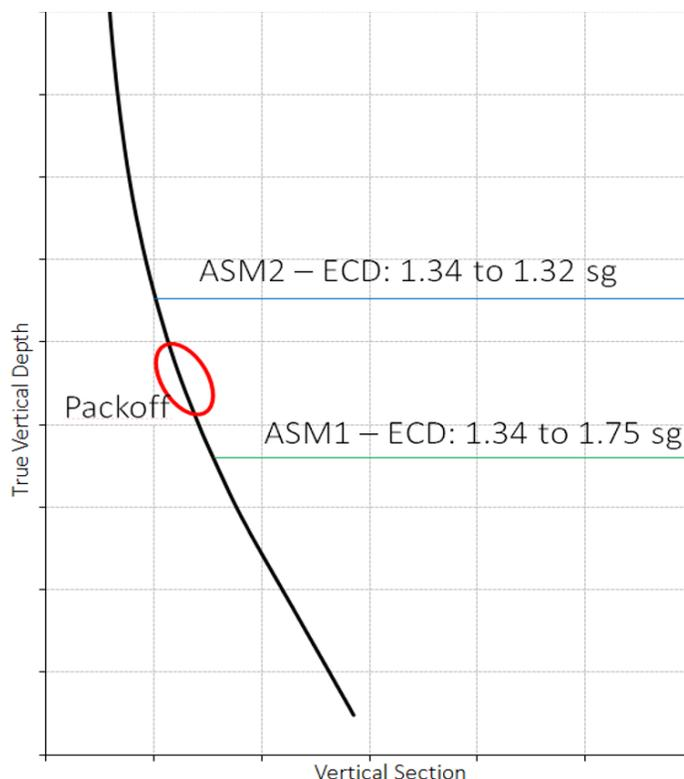
**Figure 1** – This trajectory profile highlights how the ECD measurements along the string provided by the BlackStream ASM tools changed when the packoff was seen. These helped determine where drillpipe was stuck.
